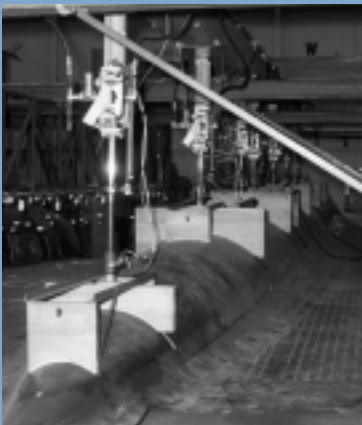
Early position transducer use: YF-12 aircraft dynamic testing in 1970.
