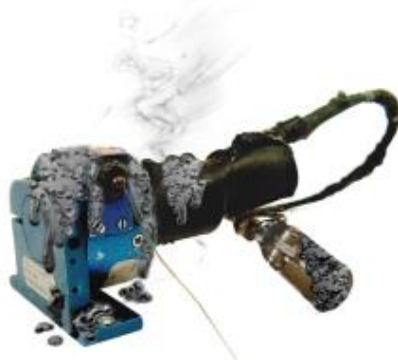
Figure 6 - Even after a high-speed collision during a NASCAR practice lap, Firstmark Controls position transducers are still intact.
