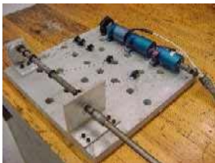
Battle tested: series of 5 position transducers after going through the DO-160D / ED-14D environmental test suite
